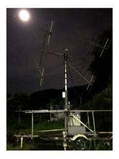
My first EME contest, Antenna: 4 x 9 V-pol Yagi Power: 300 W Rig: Icom IC-746 OP name: Huawei Su OP Callsign: BX2AI OP Grid: PL05SA
